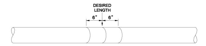
Use a fine-tooth carpenters handsaw or PVC saw to cut the PVC or HDPE casing. Remove the casing and cut off the insulation. Be careful not to damage ductile iron carrier pipe during this operation. See illustration below.
