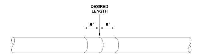
Use a carpenter handsaw or PVC saw to cut the PVC or HDPE casing. Be careful not to damage the FRP carrier pipe during this cutting operation. Remove the casing and cut off the insulation. See illustration below.
