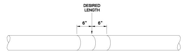
Use a carpenters handsaw or PVC saw to cut the PVC or HDPE casing. Remove the casing and cut off the insulation. Be careful not to damage steel carrier pipe during this operation. See illustration below.
