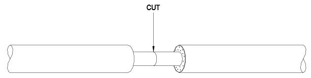
Mark, cut, and bevel the steel pipe at the desired length. Make sure cut is square. Remove any burrs and ridges on the pipe. Using a utility knife, remove the insulation between the casing and the carrier pipe one inch in from the face of the casing as shown below. Insert the rubber end seal between the casing and the carrier pipe using the handle of a hammer or screwdriver to push the seal all the way. Silicone caulking may be used in lieu of the rubber end seal.
